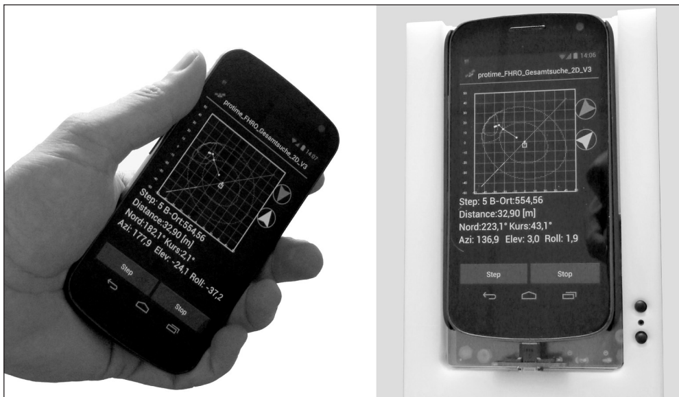
An extra piece of hardware coupled with the LawinenFon app transforms any smartphone into an avalanche transceiver. Pictured: the Galileo-LawinenFon prototype. (© Fraunhofer IML) | Picture in color and printing quality: www.fraunhofer.de/press
