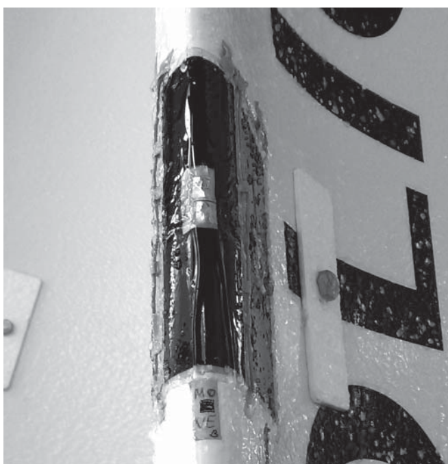
The area on the rotor blade heated by the CNT-coating remains free of ice. (© Fraunhofer IPA) | Picture in color and printing quality: www.fraunhofer.de/press
