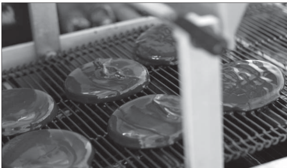
On the conveyor belt, chocolate-coated wafers are moved through the cooling channel. (© Fraunhofer IVV) | Picture in color and printing quality: www.fraunhofer.de/press
