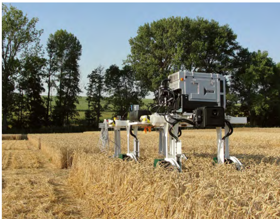
Field robot DeBiFix examines entire wheat fields to show how the kernels are developing inside the ears.
